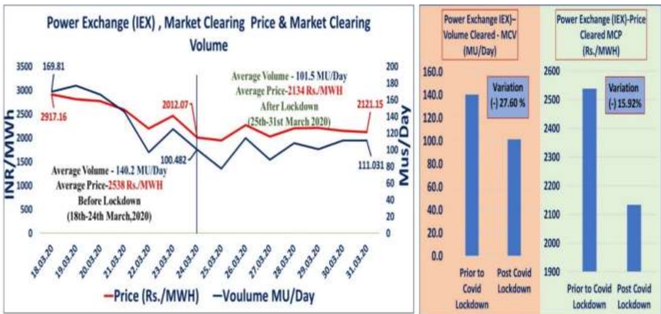
Figure 13 Power Exchange: Market Clearing Volume & Market Clearing Price (MCP) & average drop in MCV and MCP during Pre and Post COVID-19 lockdown [26]
